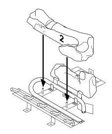
Figure 54 - Installing Log No. 2
